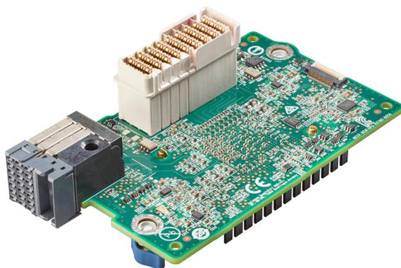
**Figure 8-2:** HPE Synergy 3820C 10/20 Gb Converged Network Adapter.
